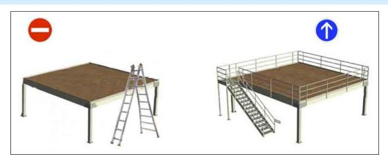
The company in charge of the building and dismantling of the double decker marquee, a mezzanine, a stage, a grandstand, a structure, etc ... must put in place for the delivery access a system that provides, at anytime, a collective protection for the people working at height at all times (materials storage area, ramp equipped with protections, etc ....
